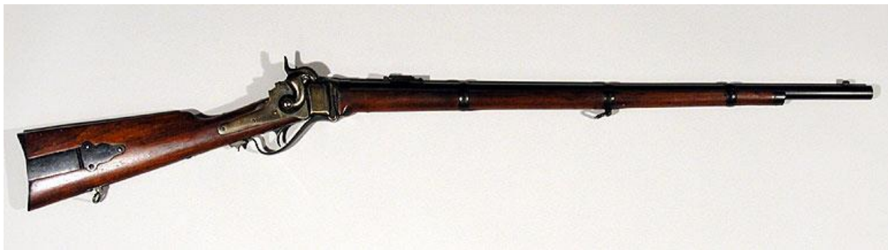
Figure 4 A Sharps Breech Loading Rifle (Note the lack of a ramrod beneath the barrel)
